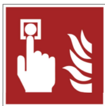
F005 Fire alarm call point
