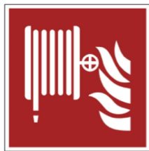
F002 Fire hose reel
