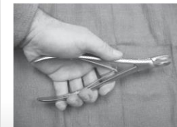
FIGURE 16.34 Grip span during use of a surgical instrument. FIGURE 16.35 Grip force exerted as a function of grip opening. (Salvendy, G. Handbook of Human Factors and Ergonomics (2nd ed.), Reprinted from John Wiley & Sons, Inc. With permission.)
